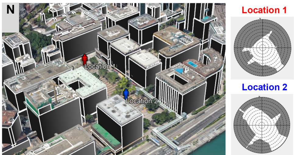
Fig. 2 Demonstration of the skymask based on the 3D building model corresponding to different locations. The skymask (right) indicates the sky view with the building blockage (gray area) projected by the corresponding building models on Google Earth (left)
